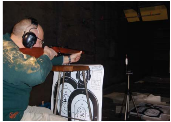
Photo2. Demonstration of shooting from a distance of 1m from the end of the barrel of a firearm.
